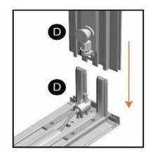
3. Matching letter stickers, attach each lower vertical pieces to the frame base. The power connections will be made automatically.
