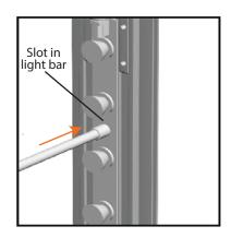
6. Insert the frame center support pole into the slots to keep the frame sides straight.
