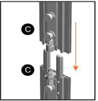
4. Attach the two upper vertical pieces to the corresponding lower vertical pieces.
