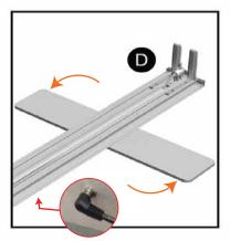
2A. Swivel the two feet on the bottom of the frame base.
