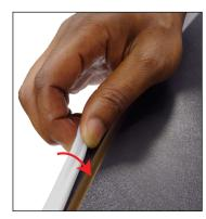
6. Fold and tuck the silicone edge into the channel. Flip the counter and repeat.
